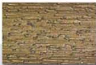
Diamond type S Less pull-out due to coating effects
