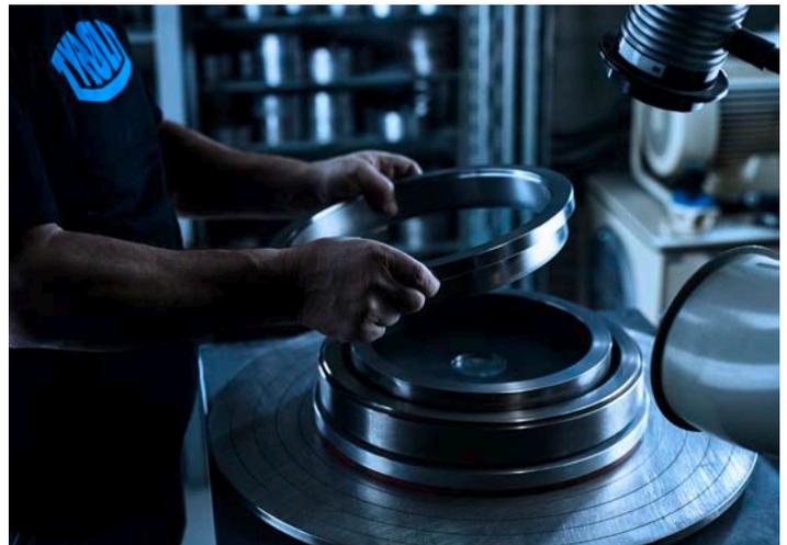
Calibrating, squaring and chamfering wheels
