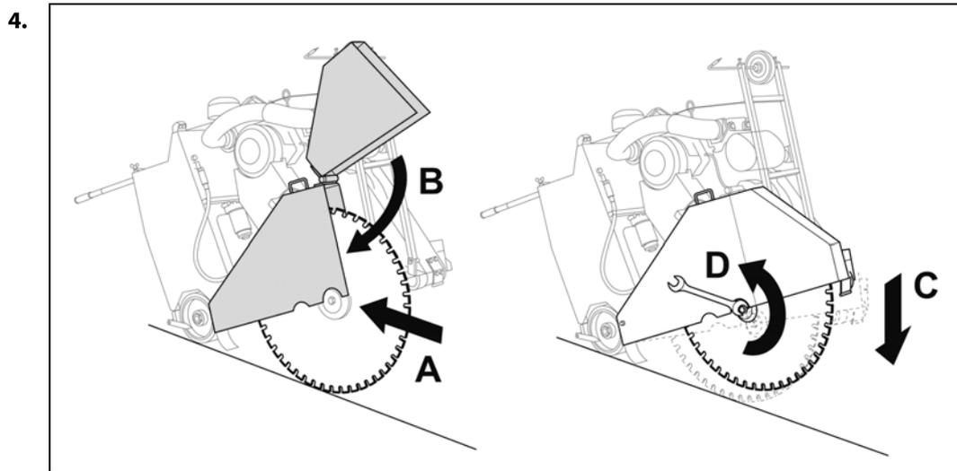
C: To prevent the saw blade rotating while being tightened, carefully place the saw blade on the floor.
