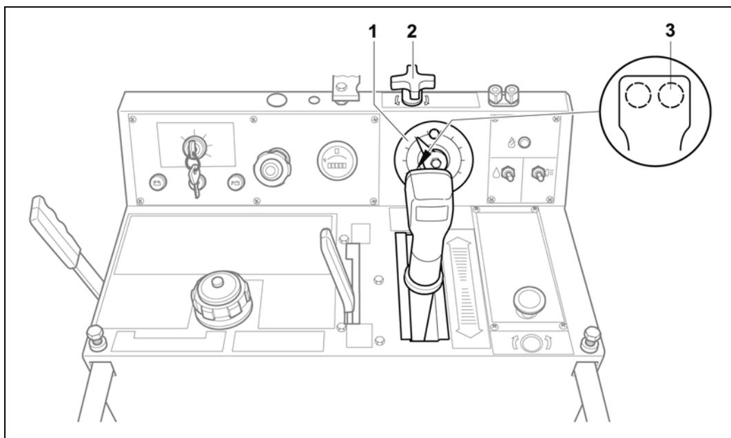
1. Press the **Lower** button (3) until the saw blade touches the material to be cut.
